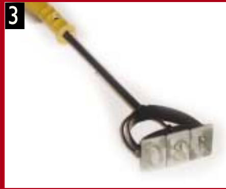
3 Brand for at least 15sec. & put back to heating position
